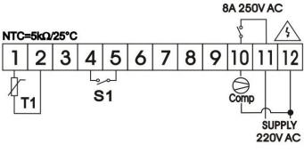
T1:Temperature Sensor S1:External Alarm Signal
